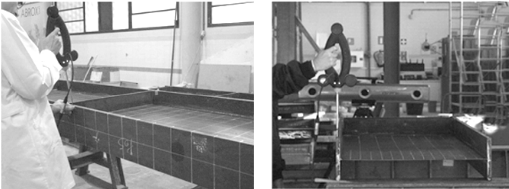
Figure 3.10. Measurement of initial imperfections.
